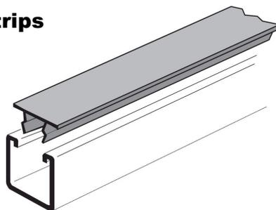
Elevator Guide Rail Insert Closure Strips, or snap-in covers, keep construction debris out. Exceptionally useful during inserts installation in masonry wall. Dark grey color, PVC, 1-3/8" wide, 1/16" thick.
